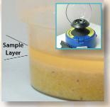
3. Corn: Allow to settle into two layers (sample taken from top layer). Corn flour: centrifuge 1 min.
