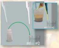
4. Using pipette and new tip, add 1.5 mL of DB6 Buffer to the first vial (dilution vial); then using the MiniPet and new tip, add 200 μL extract to the first vial. Mix by pipetting up and down 5-10 times.
