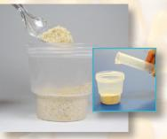
1. Add a 20 to 50 gram sub-sample to container, then add 5 mL of water\* per gram of sample
