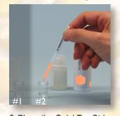
6. Place the QuickTox Strip in the reaction vial; wait 5 minutes for results
