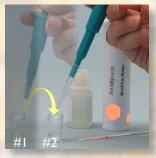
5. Transfer 200 µL of the mixed sample from the first vial (dilution vial) into the second vial (reaction vial)
