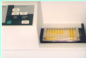
Read plates in a Plate Reader within 30 minutes of the addition of Stop Solution
