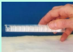
Slap inverted plate on towel to remove as much liquid as possible
