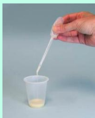
Transfer extract to cup, about 3 pipettefuls
