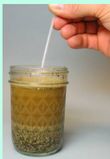
Avoid pulling up particles when drawing sample
