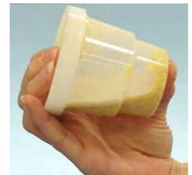
3. Shake immediately for 10 seconds to dissolve the pouch, then for 1 minute on a mechanical shaker or 2 minutes by hand
