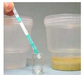
6. Place the QuickTox strip in the vial, wait 4 minutes. Remove strip immediately and interpret.
