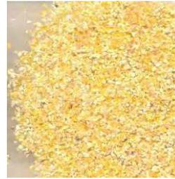
Example of a sample ground too coarse which will result in improper extraction – INCORRECT
