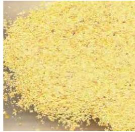
Collect and grind a representative corn sample such that 95% passes through a 20-mesh sieve - CORRECT
