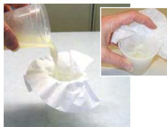
4. Filter the sample into a clean vessel with an approved coffee filter; move the filter to the side to access filtered extract
