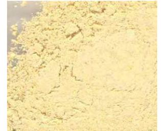
Example of a sample ground too fine which will impede the flow of extract up the strip – INCORRECT
