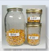
Determine sample weight and place in properly sized jar
