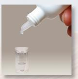
3. Set sample extract down to settle, meanwhile add one drop 1N HCl to reaction vial
