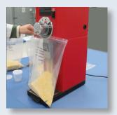
Alternately, grind with coffee grinder
