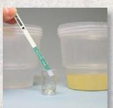
6. Stir <u>well</u> with pipette, then add test strip; wait <u>5 minutes</u> for results
