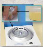
4. Centrifuge a portion of extract for **1 minute** at 2000 x g (NOT RPM).
