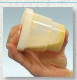
3. Shake 1 minute on mechanical shaker or by hand for 2 minutes
