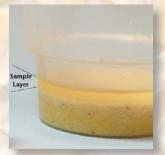
4. Allow to settle into two layers - top layer is where sample is taken
