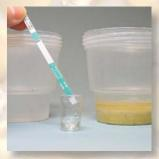
6. Stir well with pipette and add test strip, wait 5 minutes for results
