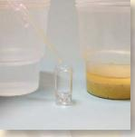
5. Add one pipette of tap water to vial first, then one from sample
