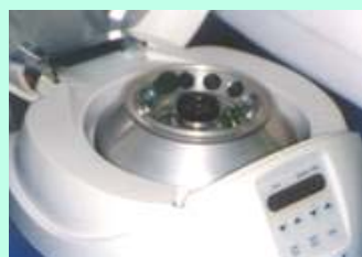
Centrifuge to clarify grain extract
