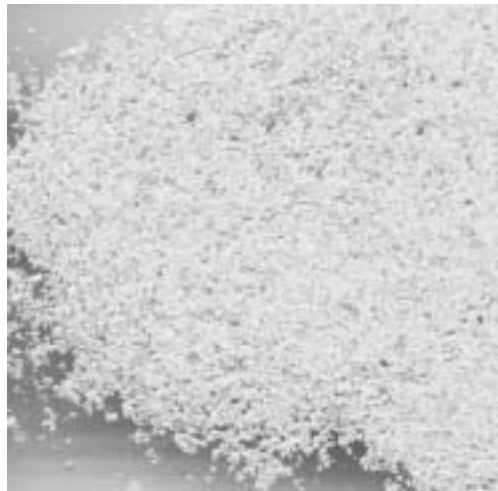
Correct 20 mesh grind
