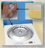
4. Centrifuge a portion of extract for 1 minute at 2000 x q (NOT RPM).
