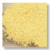
1. Collect and grind representative sample such that ≥95% passes through a 20 mesh sieve
