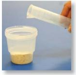
3. Add 5 mL/g of distilled, deionized, or bottled water (eg: 250 mL for 50g sample)
