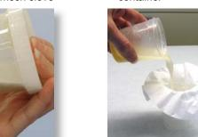
5. Filter extract using approved coffee filter into a clean vessel
