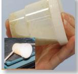
4. Seal/cover container and shake on mechanical shaker (or vigorously by hand) for 30 seconds
