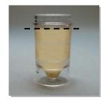
Measure water using the Soybean Common Extraction™ (5 mL water per gram of sample). For example, you want to test 400 beans with an average weight of .15g;  $400 \times .15 = a 60 \text{ g sample}$ x 5 mL/g = 300 mL water). Add to container, cover and shake to wet entire sample.
